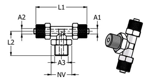
Hose diameter A1 = 8/6Hose diameter A1 = -Hose diameter A2 = 8/6L1 = 40L2 = 27.5NV = 16Thread A3 = G 1/4"
